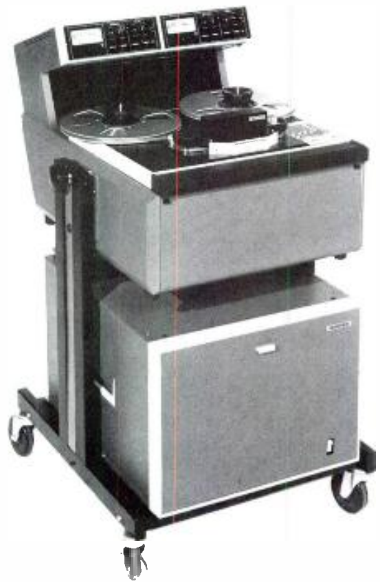
Figure 10. An Ampex digital prototype, offering four channels on quarter-inch tape (50 kHz sampling rate). A series of experimental sessions are planned for later this year.
