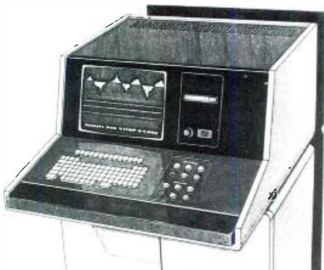
Figure 1. An artist's conception of an early 3M editing system. When pre-production prototypes were judged overly complex for routine editing chores, the system seen in Figure 2 was developed.
