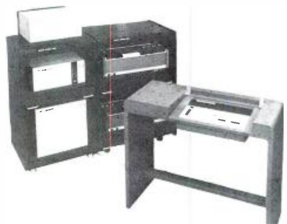
Figure 5. JVC Series 90 Digital Audio Mastering System, incorporating video tape recorders.
