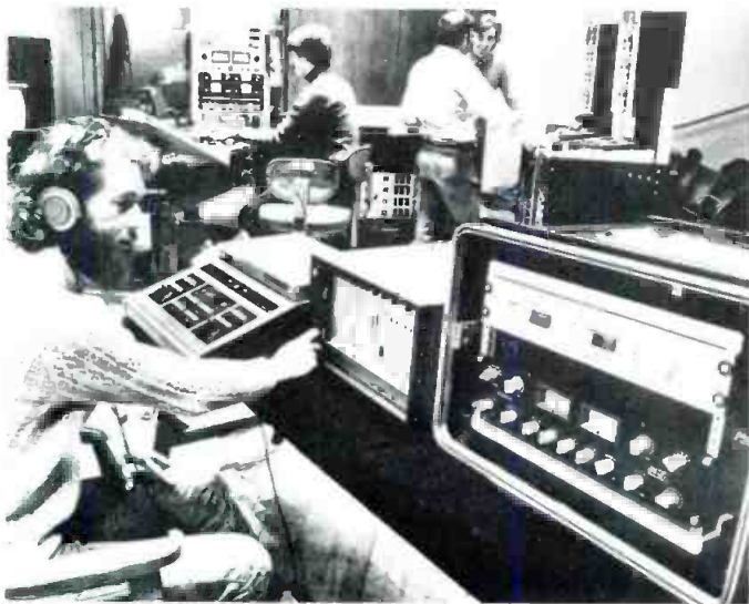
Figure 7. Peter Jensen of Digital Recording Systems at a Metropolitan Opera recording session. In front of him are: Sony's BVE-500A editing console, a Sony PCM-1600 Digital Processor, and a Mark Levinson preamplifier.
